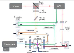
**Fig. 1**. Experimental CARS setup. OPA: optical parametric amplifier, IF: interferential filter, L1, L2: lenses, CCD: charge coupled device.
